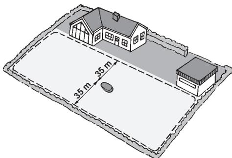
When the Auto Mower's working area borders, e.g. collections of water, driveways and pathways, etc. the boundary wire should be supplemented with a number of posts, edging or a fence with a height of at least 15 cm. This is an additional safety measure to prevent the Auto Mower from running outside of its working area if the boundary wire is installed incorrectly.
