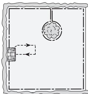
The boundary wire must be no longer than 500 metres. The distance between the Auto Mower and the nearest part of the boundary wire must not exceed 35 meters anywhere in the working area.
