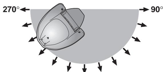
The mower normally leaves the charging station at a random angle within the range 90–270° (see diagram).
