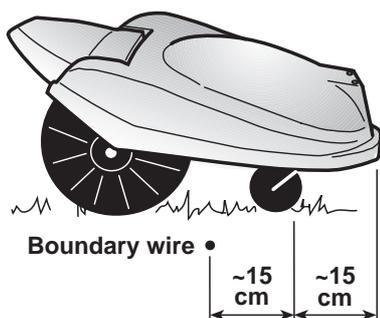
How far inside the outer edge of the working area the boundary wire should be placed depends on what lies immediately outside the area. If there is a high obstacle, such as a wall or fence, or delicate flowers, just outside the area to be mown, the boundary wire should be laid 40 cm from the obstacle. This should prevent the Auto Mower bumping into it.
