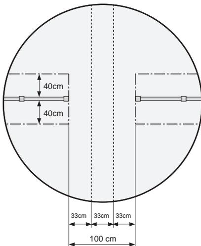
Since the Auto Mower follows the path of the search wire, it must be laid at least 40 cm away from any obstacle to prevent the Auto Mower from bumping into anything on its way to the charging station.
