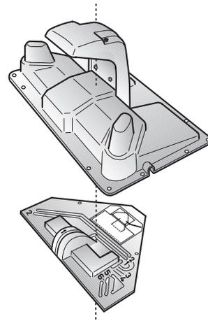
The incoming ends of the boundary wires are routed through the slots in the lower section. The docking unit is then placed over the lower section. NOTE! To ensure that the Auto Mower docks correctly with the charging station it is important that the cables are actually laid in the channels in the lower section.
