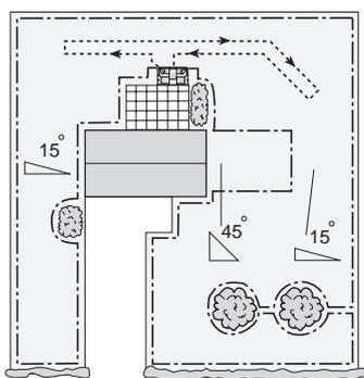
Lay out the boundary wire and secure it to the ground using staples so that there is no risk of the blades cutting the cable. Allow the Auto Mower to work for a week and then decide whether any adjustments to the wire routing are necessary. After a few weeks the grass will have "weaved in" the cable so that it is not visible. The boundary cable can also be laid 2-5 cm (maximum 20 cm) under the soil.
