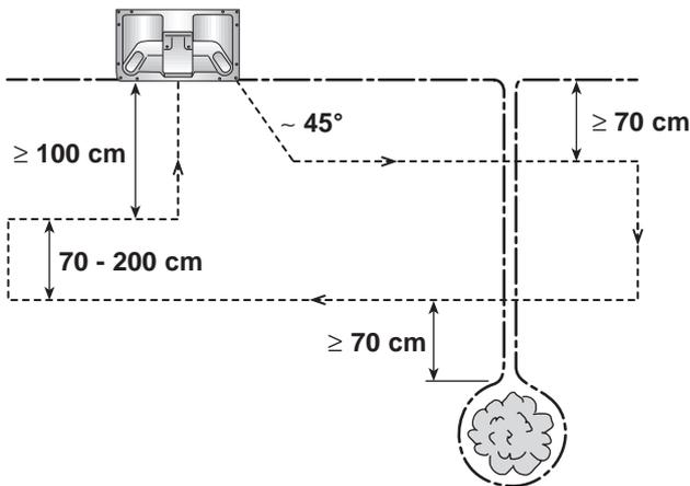
In exceptional cases and over short distances the wires can be laid closer together, i.e. in a narrow passageway or in the final metre approach to the charging station. If so, it is important that the wires are equally spaced.
