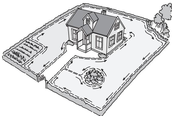
When the Auto Mower reaches the boundary wire it senses that it is passing the wire. It then continues for a short distance beyond the wire before reversing.
