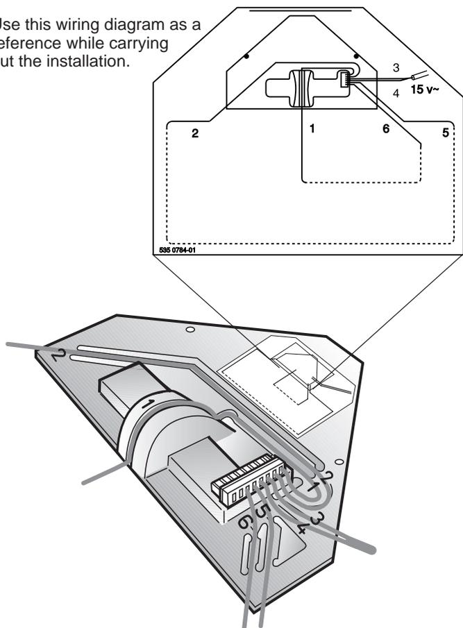
**NOTE! Do not let any metal objects touch the charging station contact plates while the transformer mains cable is plugged into the power socket. This can cause the plates to short-circuit and the transformer fuse will trip. There is no risk of harmful electric shock from the 15 V low-voltage supply.**
