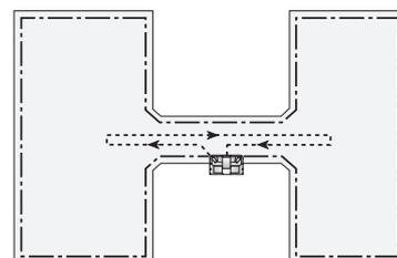
The area in front of the charging station should be as open as possible. Don't put the charging station in a "pocket". We recommend that the charging station is placed somewhere along a straight part of the boundary wire rather than in a corner.
